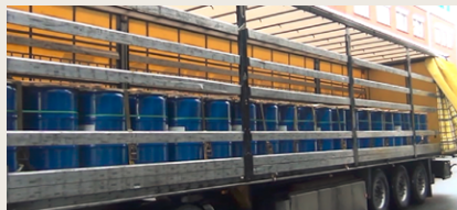
Force-locking cargo-securing by lashing down
