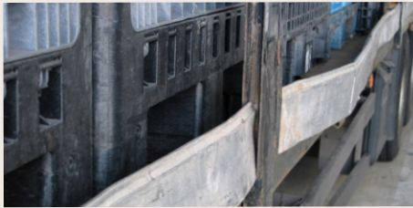
Bent lightweight metal insertable rigging boards
