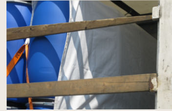
Defective/cracked wooden insertable rigging boards
