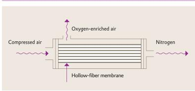
Compressed air is injected into the hollow-fiber membranes in order to separate off the nitrogen. Oxygen molecules are smaller than nitrogen molecules so they permeate the membranes more easily. The nitrogen therefore accumulates inside the hollow fiber, while oxygen accumulates on the outside.
