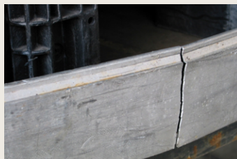
Defective lightweight metal insertable rigging boards
