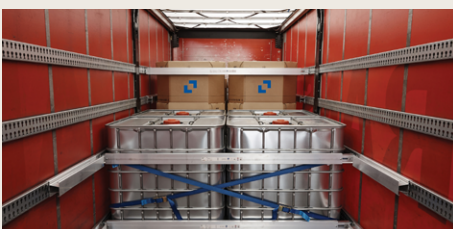
Form-locking loading with the aid of AJS-CP3 protectors
