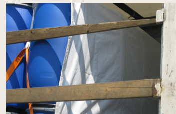
Defective/cracked wooden insertable rigging boards
