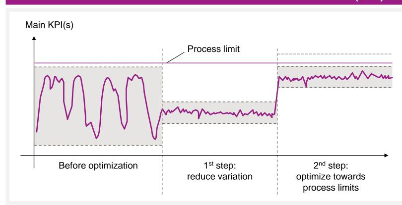
**APC optimizes** complex production processes under consideration of many process parameters and ensures production at the ideal operating point
