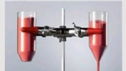
Improved flowability by hydrophobic Silica
